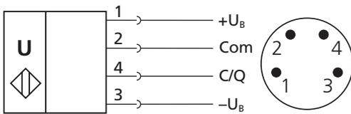
Fig. 3: Connection diagram of the pms sensor
