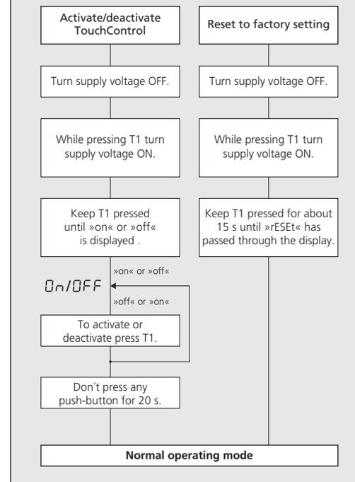
**Diagram 4: Useful additional functions in Add-on menu (for experienced users only, settings not required for standard applications)**
