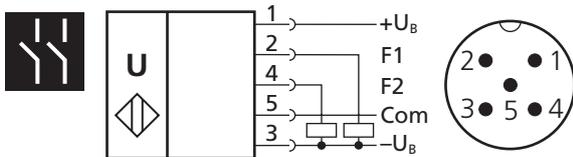
Fig. 3: Connection diagram of the ucs sensors
