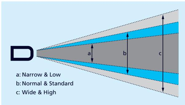
Fig. 11: Setting options for the detection zone width
