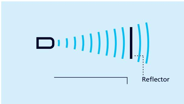
Fig. 9: Two way reflective barrier, window ± set point offset
